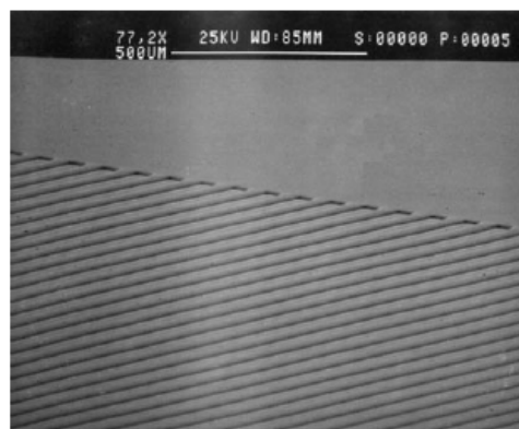
Figure 15. PMMA channels 5 \mu\text{m} deep [4]
