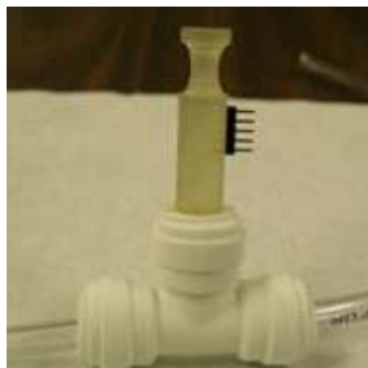
Figure 59. Type II package assembled with 3/8" standard fitting [27].
